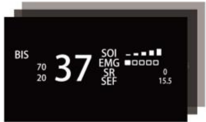
BIS (bispectral index) Used to determine the depth of sedation or induced hypnosis.
